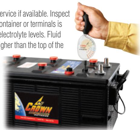
If the battery is sufficiently filled with electrolyte – proceed to step 2. If the top of the battery's plates are not covered with liquid, add water, replace vent caps and place the battery on charge. Be sure no open flame or spark is near while the battery's vent caps are removed from the battery.
